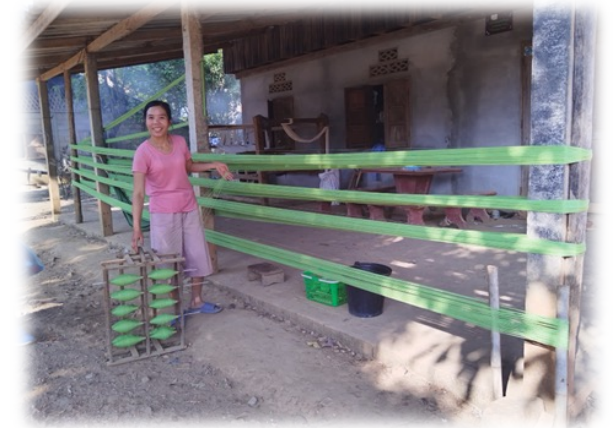
Prepare cotton threads are long enough for the size of fabric you want to weave.
